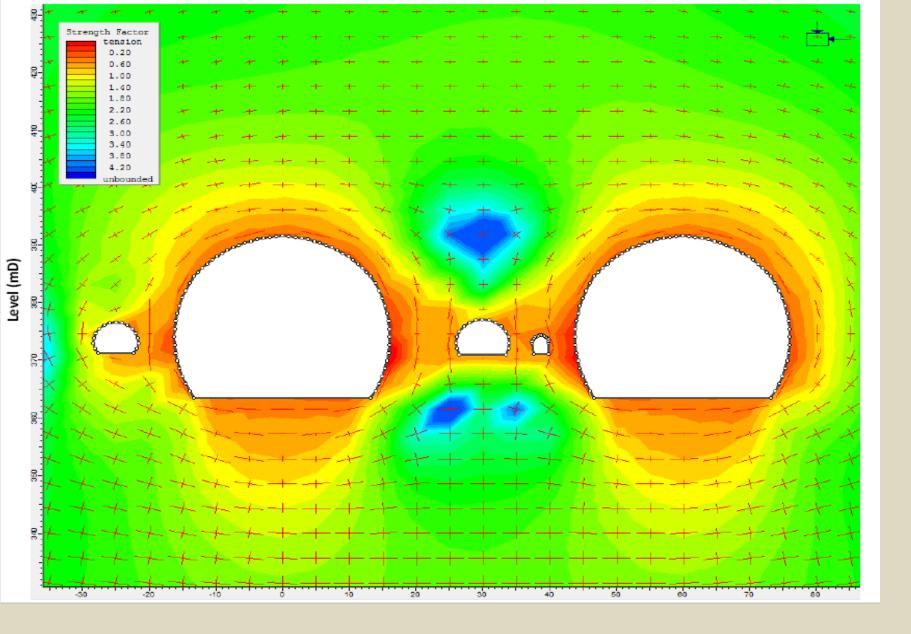
2d and 3d models will be developed for CLIC to do a "Time-dependant" state analysis. Possible 2<sup>nd</sup> phase use of these models for ILC layouts/geology.
