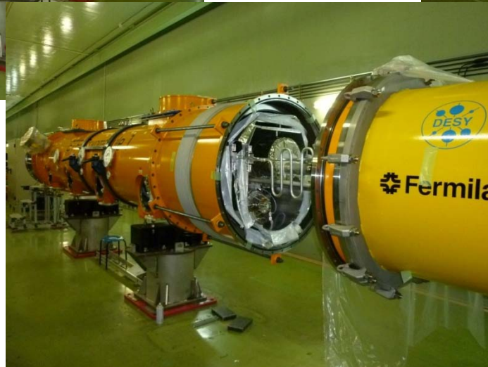
Connection between Cryomodule-A and -C
