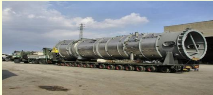
Oxychlorination reactor -Cladded material Dimension Dia. 4,1 m X L. 20m , 165 Tons
