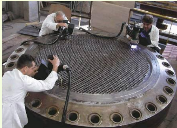
Orbital welding of heat exchanger tubesheet Material S.S. And Zirconium
