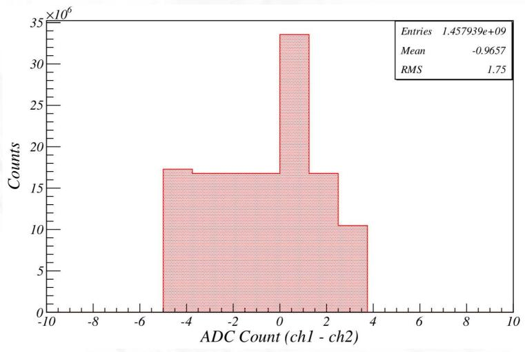
Pedestal difference between two channel in one ASIC.
