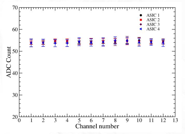
Pedestal for 4 ASIC and each has 12 channel (example)
