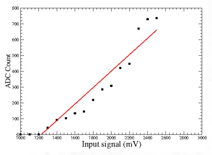
Not ideal linearity, but ADC functional for different injected charge
