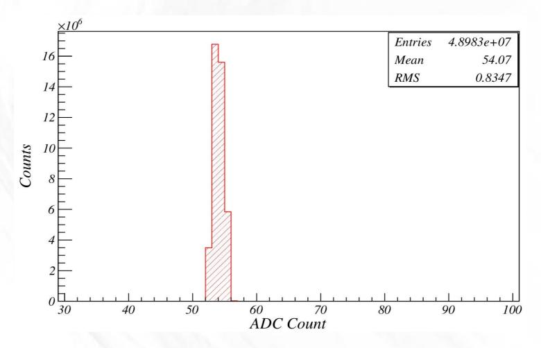
Pedestal for 1 channel in one ASIC, the mean value is around 54 ADC Count or 1.2 MIP (1 MIP = 45 ADC Count)
