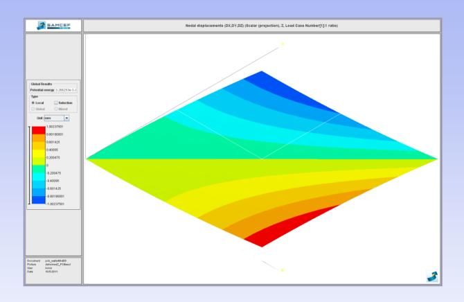
Deformations of ¼ shell PCB (2 symmetries applied). Maximale Deflection was 1mm.
