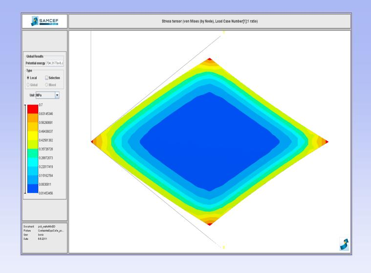
Von Mises Equivalent Stress in Glue Max stress = 0.7MPa
