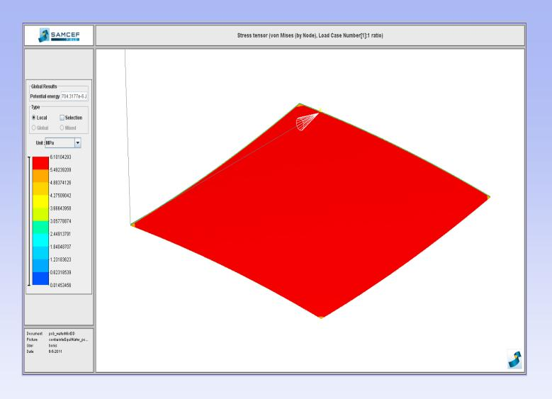
Von Mises Equivalent Stress in wafer Max stress = 6.1MPa
