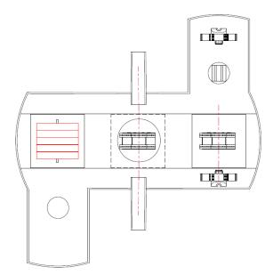
Single Gantry Serviced Shaft for Detector Subcomponents with smaller service shafts serviced by above ground crane
