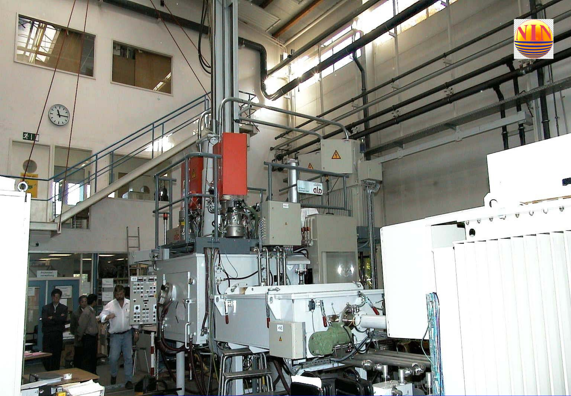
500KW electron beam cold hearth furnace
