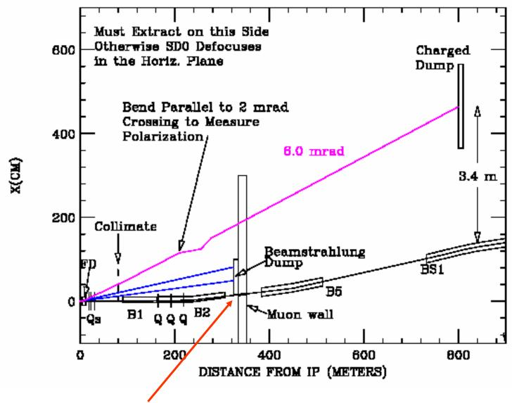
Note proximity of beamstrahlung dump to the incoming beam – may need to put the incoming beam line pipe through the water tank.
