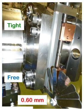
Measurement of thickness gauge
