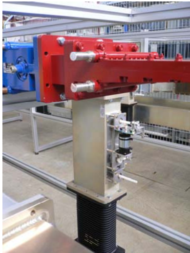
Phase shifter replaced with 3 stub tuner. One motor drive is enough.
