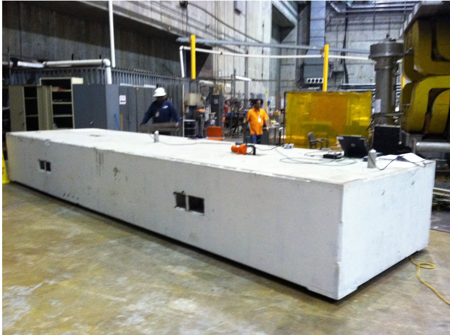
Vibrator and Sensors on Block
