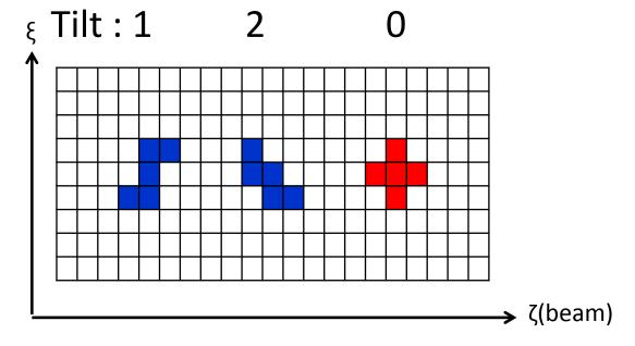
Filtering performance is being checked by using this cluster shape information. ("tilt" was not be used in previous study.)
