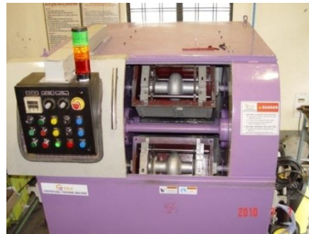
Centrifugal barrel polishing machine developed
