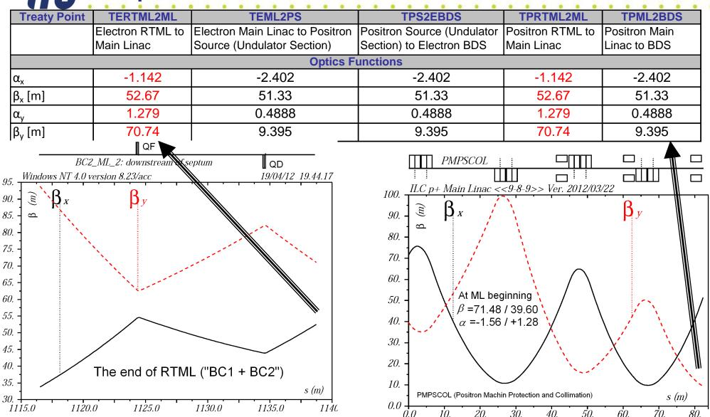
Actually ML ends at the entry of PMSCOL (p+ machine protection & collimation )
