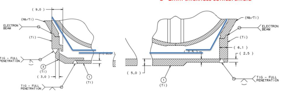
Conical shield can be formed by press and put into endplate during end-group welding
