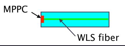
plastic scintillator 10mm x 45 mm x 3mm 1mmΦ WLS fiber
