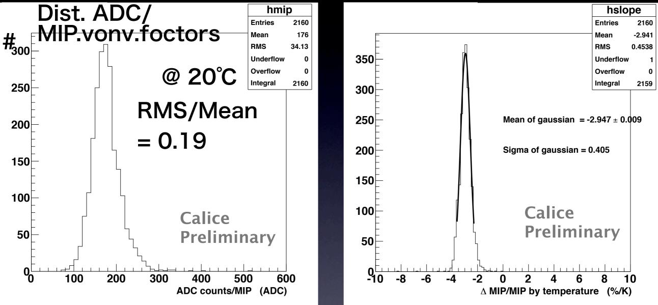
Variation of ADC/MIP.conv.factor is 19%, ▶ This comes from Scintillator WLS fiber system (variations of scintillator quality, MPPC fiber miss matching and so on.) ∵ Variation of MPPC gains is less than a few%
