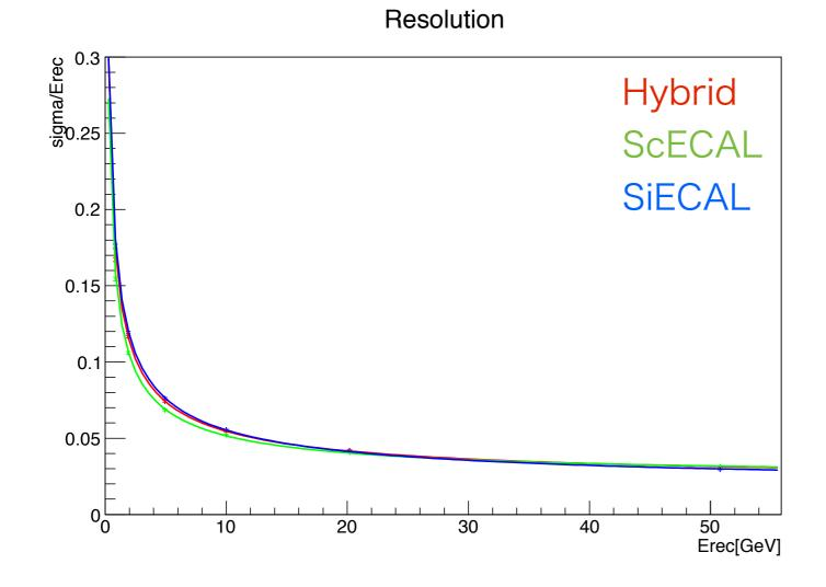
$$\frac{\sigma}{E_{Rec}} = \sqrt{\frac{\left(\sigma_{stoc.}\right)^2}{E_{Rec}} + \left(\sigma_{const.}\right)^2}$$
