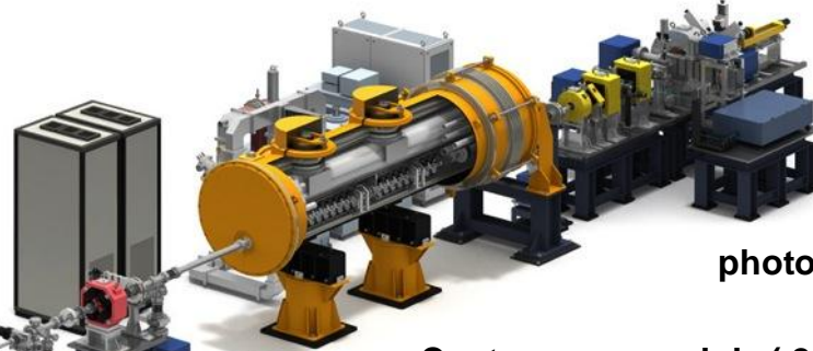
Capture cryomodule ( 2 SC cavities )
