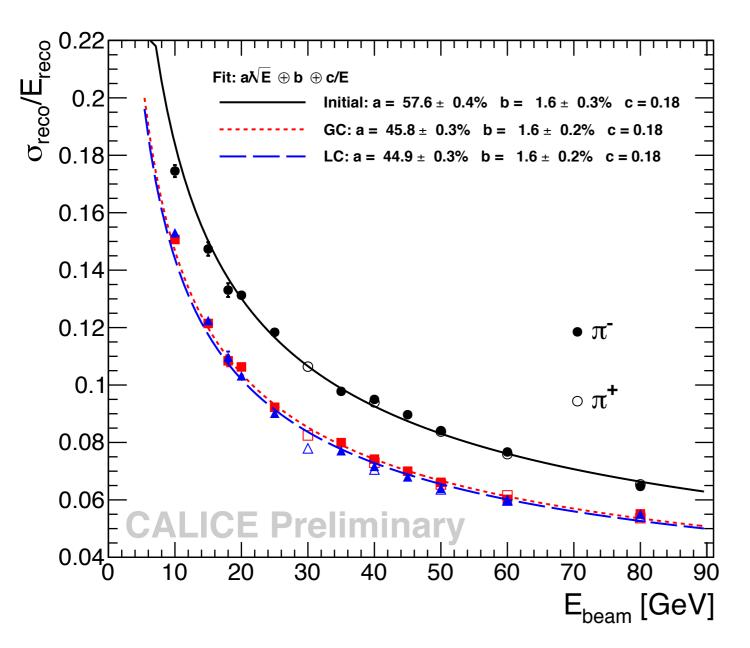
Resolution of 45%/VE with small constant term for pions *in data*Linear energy reconstruction within 1.5% over the full energy range from 10 GeV to 80 GeV
