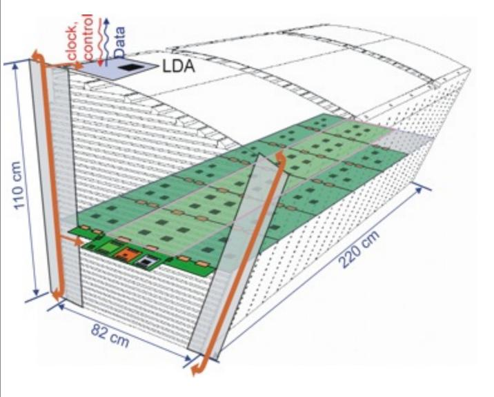
compact construction: Minimized gaps, ASICs embedded in PCB Indivdual electronic boards (HBUs)
