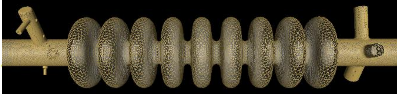
FNAL 3.9GHz 9-cell cavity in Omega3p. K.Ko, et al
