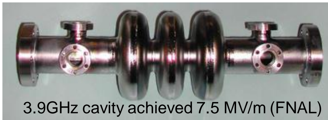
FNAL 3.9GHz 9-cell cavity in Omega3p. K.Ko, et al
