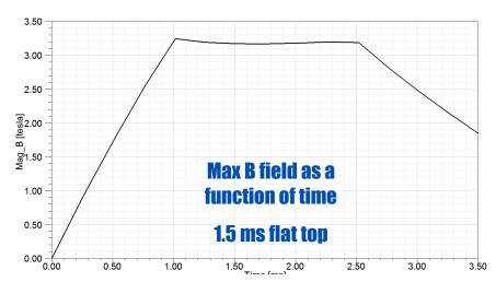
A current ramp from the pulse forming network can counteract the magnetic field droop - even at room temperature
