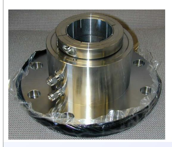
Since it seemed that we had a heating problem with the Rigaku seal we chose a lower viscosity / higher outgassing ferrofluid.
