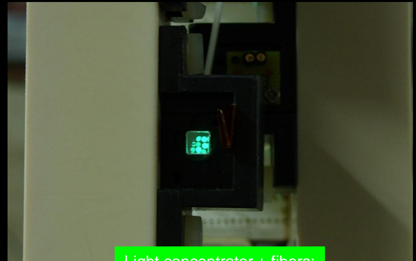
Light concentrator + fibers: SiPM side
