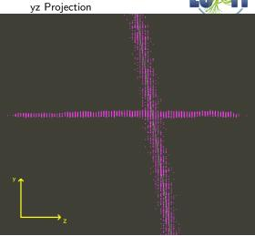
Binning in z due to 40 MHz readout frequency  $\stackrel{\scriptscriptstyle }{=} 2 \text{ mm}$  drift distance
