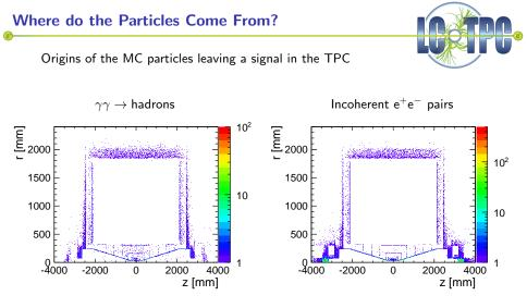
Backscattered particles from all over the detector
