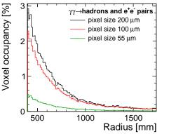
• Factor 4 in voxel occupancy between 55  $\mu$ m and 100  $\mu$ m pixels  $\Rightarrow$  Each voxel is only occupied by one electron / cluster
