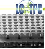
Timepix chip with integrated micro mesh
