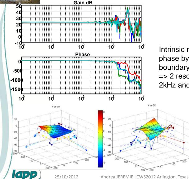
Intrinsic resonances if change of phase by 90°: other peaks just from boundary conditions => 2 resonance peaks just below 2kHz and near 4kHz.
