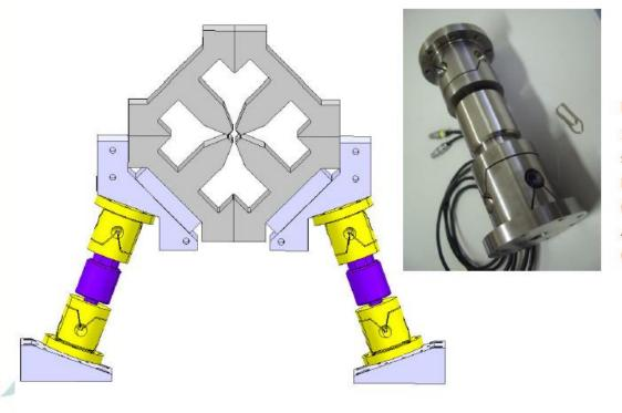
Universal Flexural Joint 2 rotation axes in the same plane rotational stiffness (k<sub>e</sub>=220Nm/rad) Axial stiffness (k<sub>aj</sub>=300N/µm)
