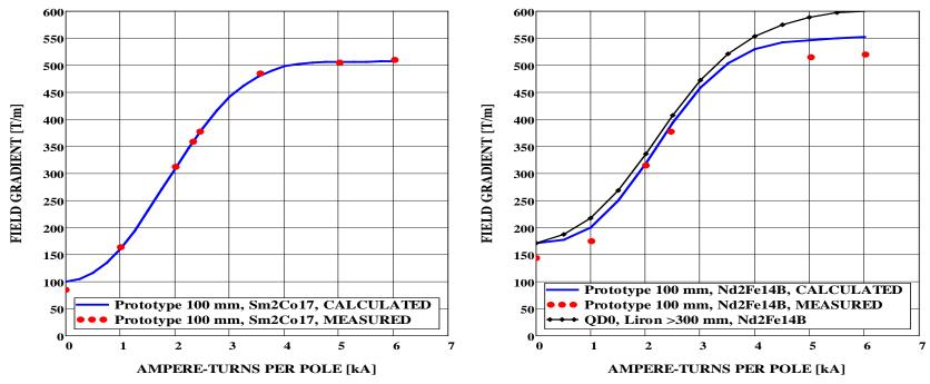
The measured Gradient in the configuration with  $Sm_2Co_{17}$  blocks (left) is in very good agreement with the FEA computation. This is not the case for the  $Nd_2Fe_{14}B$  blocks (rigth) were a difference of ~ - 6% at maximum gradient is visible. This could have 2 possible explanation (the 1<sup>st</sup> was excluded by a further FEA cross-check):
