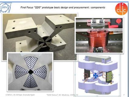
Activities going on in 2012 and magnet was finally assembled and tested in two configuration: with  $Nd_2Fe_{14}B$  and with  $Sm_2Co_{17}$ permanent magnet blocks.
