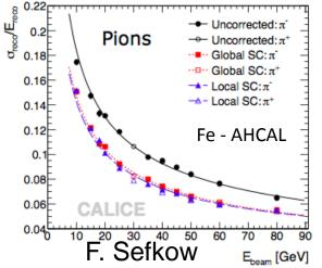
Local compensation: re-weighting based on single cell energy density
