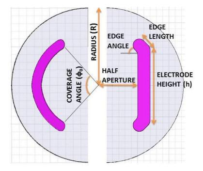
In the optimization process, we must try to reduce the capacitance between both striplines in order to achieve odd and even mode characteristic impedance close to 50  $\Omega$ . We can find three different situations:
