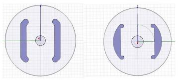
A small stripline beam pipe radius results in closer values of even and odd mode characteristic impedances.
