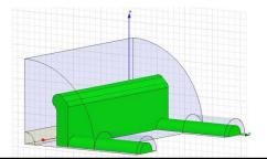
HFSShasbeenusedtocalculatethereflectionparameter $S_{11}$ looking into aninputportwhenthecorrespondingoutputportresistivelyterminated at 50 Ω.
