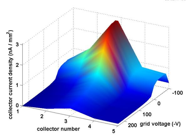
Collector steady-state current density vs retarding voltage (Cu chamber,  $I_{beam} = 56 \text{ mA}$ )
