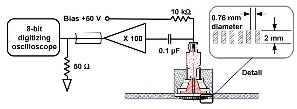
The pickup electrodes are shielded by the vacuum chamber hole pattern against the beam-induced signal.
