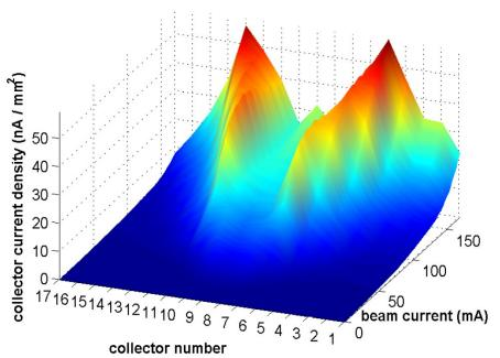
The RFA signal is sensitive to cloud photoelectrons and secondary electrons produced on the vacuum chamber wall near the vertical plane containing the beam.
