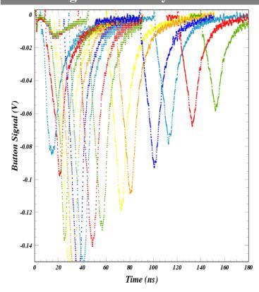
The single bunch signal arises from photoelectrons produced on the bottom of the vacuum chamber. Its shape is closely related to the photoelectron kinetic energy distribution and the beam kick. The witness bunch signal includes the single-bunch signal as well as the that produced by cloud particles accelerated into the shielded pickup by the kick from the witness bunch. The witness signal is therefore sensitive to SEY.
