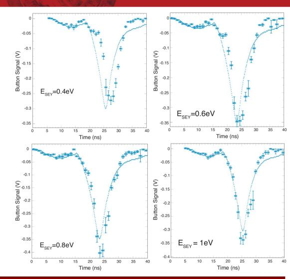
The pulse shape for the 14-ns witness bunch signal sets a lower bound on the model parameter  $E_{
