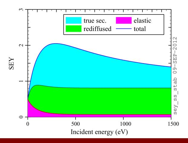
The three secondary electron yield processes differ in their dependence on incident energy and produce electrons of differing kinetic energy distributions. The relative rates of these secondary emission processes depend on the vacuum chamber surface properties such as coating, roughness, grooves, as well as on beam conditioning.
