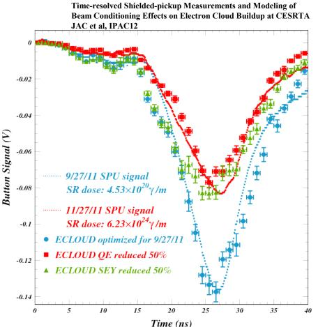
The beam conditioning effect for an amorphous carbon coating is primarily in quantum efficiency in both the early and late conditioning processes.
