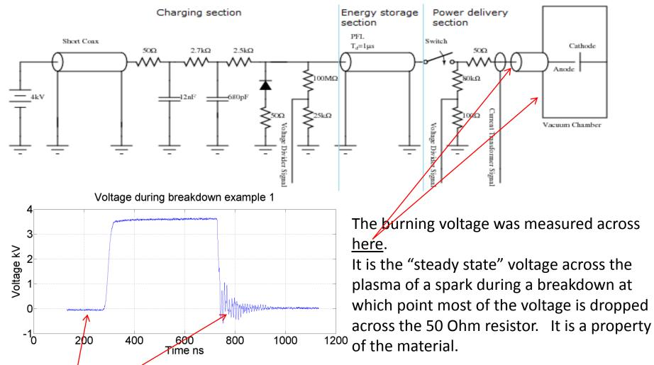
Subtract average voltage with switch closed from Average voltage during breakdown after initial voltage fall.
