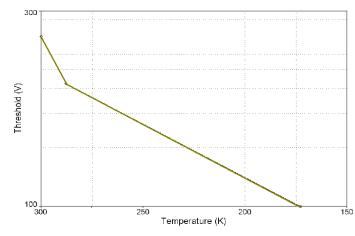
Arc threshold vs. sample temperature
