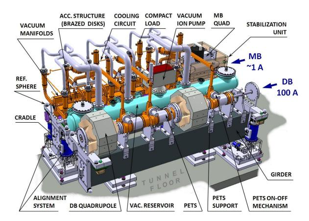
CLIC at 500 GeV (4'232 modules) 26'920 Accelerating Structures 13'460 PETS ~ 70'000 RF components CLIC at 1.5 TeV (10'730 modules) 71'380 Accelerating Structures 35'690 PETS ~ 200'000 RF components
