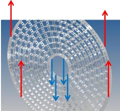
Endplate is supported at 4 points (*red arrows*) upper points are constraints, right fixed, left sliding lower points are forces
