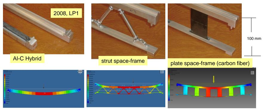
(Carbon fiber material is specified to have the same rigidity as the aluminum and is treated as aluminum in the FEA.
