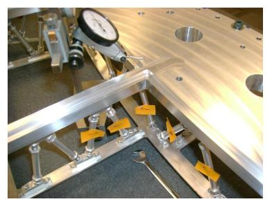
The strut design allows alignment correction.
