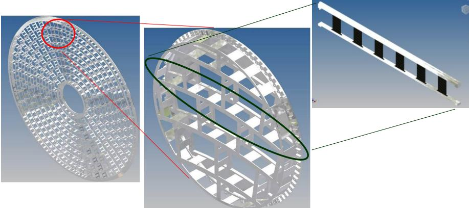
The ILD endplate design study involves endplates at 3 levels of scale. The LP1 and LP2 endplates represent small sub-sections of an ILD endplate. Small test beams represent a slice through the LP1 or LP2 endplates.
