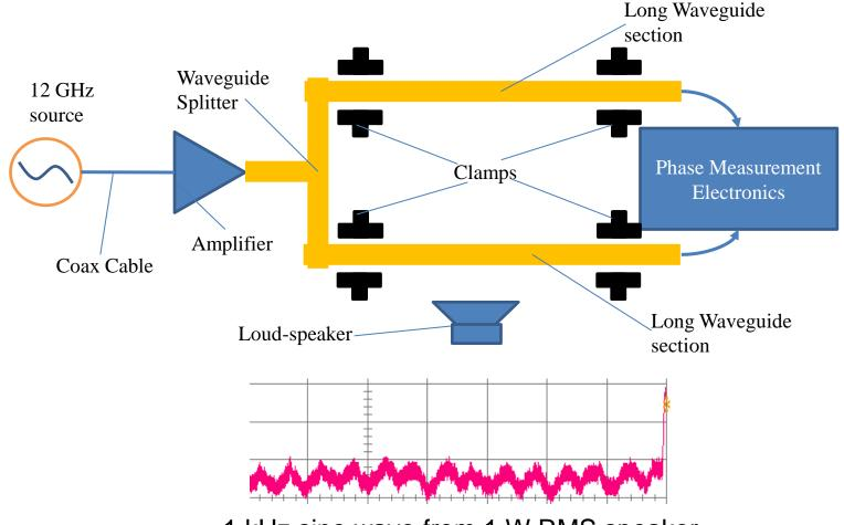
1 kHz sine wave from 1 W RMS speaker detected as a 25 milli-degree pk-pk phase variation.
