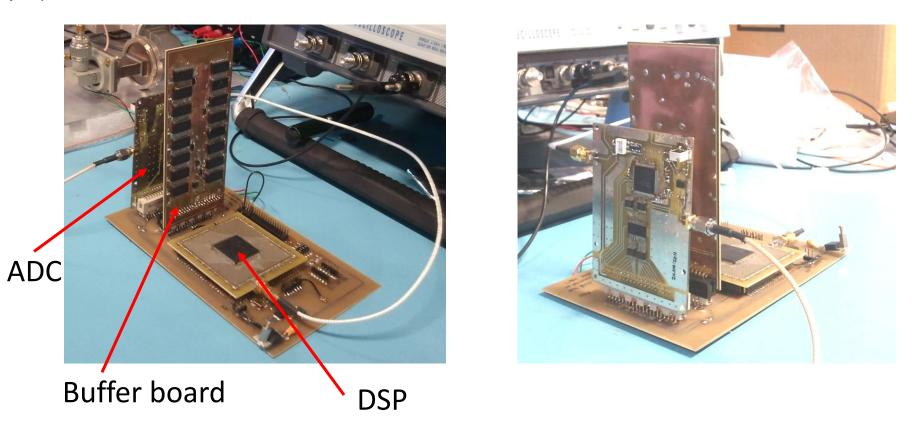
System has been manufactured and implemented with 13 noise free bits. Multiplexer is available for increased I/O.
