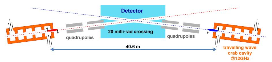
Bunches pass through deflecting cavities phased to give zero kick for bunch centres A deflecting cavity phased in this way is called a crab cavity
