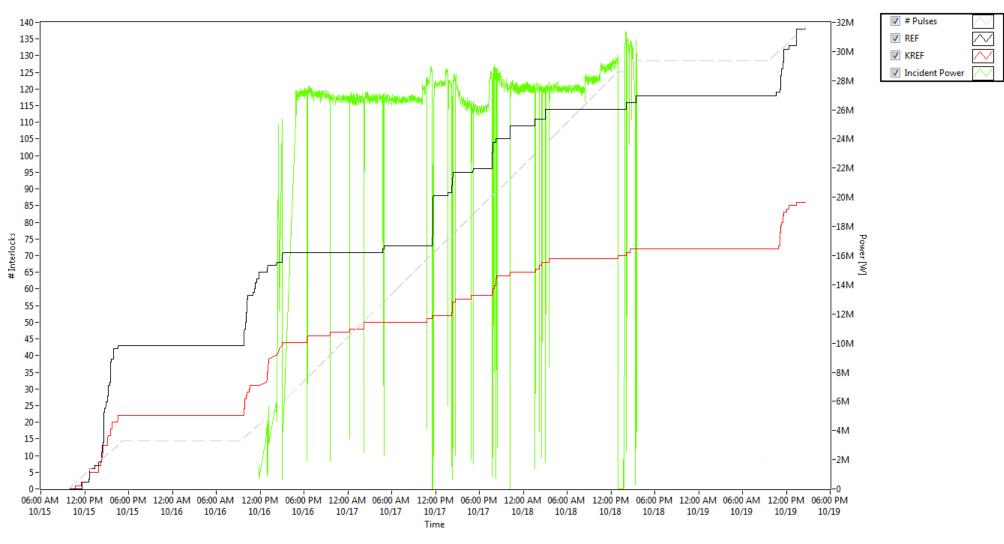
In real time, several hours of running missing due to instable pulse compressor: BDs stop rf, pulse compressor cools down and detunes, compensation using frequency tuning seems to increase structure BDR
