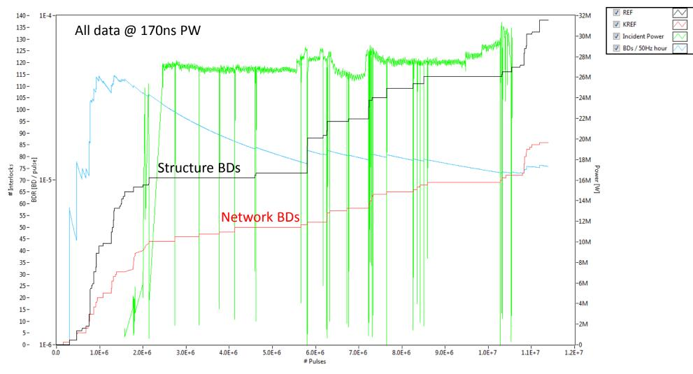
11385142 pulses (63h@50Hz), 138 structure BDs, 86 system BDs DAQ system logging deployed first time mid of October, but software development not yet completely finished! Just starting to take data!
