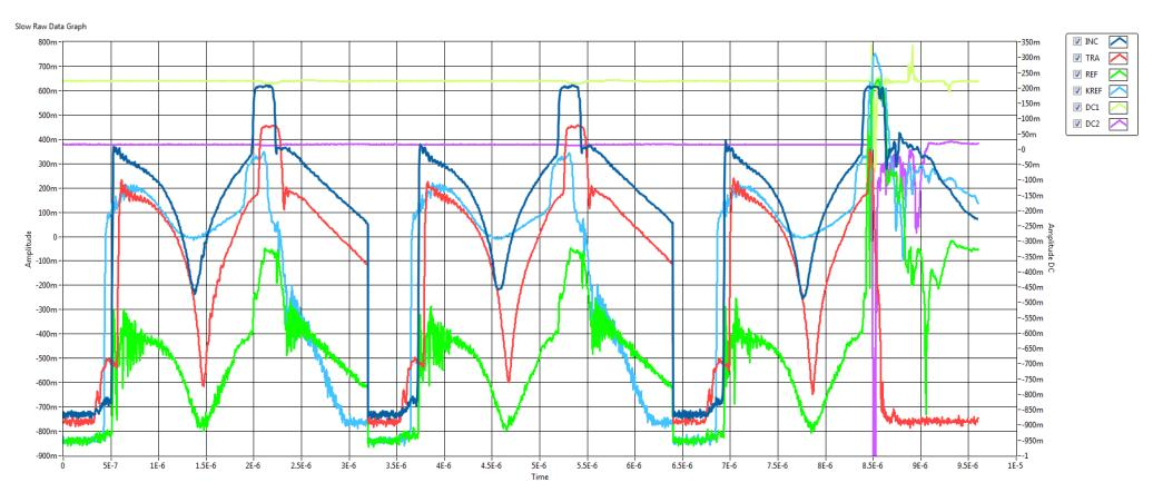
Phase modulation for pulse compression works well, rf flat top can be easily controlled using the dark current emission waveform. Logarithmic power detectors ease operation at all power levels and help to obtain good power resolution without saturation effects during breakdown.
