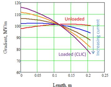
Testing of accelerating structure with nominal beam loading is a missing block in our testing program. Such a test will be done using CTF3 drive beam and RF power delivered from X-box#1 via modified 30 GHz low loss transfer line.
