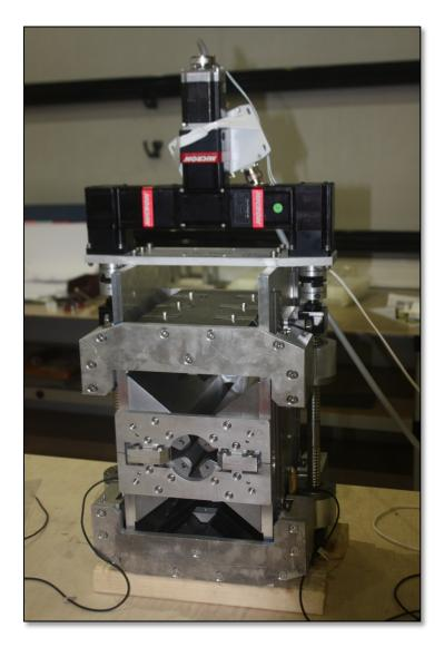
Completed Phase 1 assembly (i.e. complete assembly, commissioning of actuators, gearbox, linear encoders, etc.)
