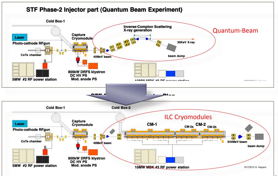
1ms bunch train with 2.5mA beam are successfully accelerated to 40MeV in Injector operation, 4 mirror laser accumulator is ready for X-ray generation experiment.
