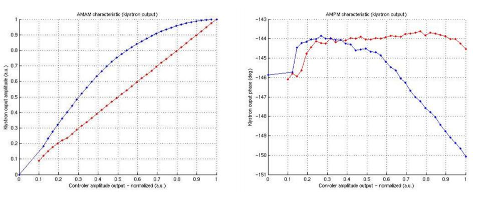
Proposed and implemented method allowed for klystron behavior linearization. Although some system weak points can be recognize (eq. poor phase detection for low signal levels) amplitude and phase characteristic correction can be considered as satisfactory.
