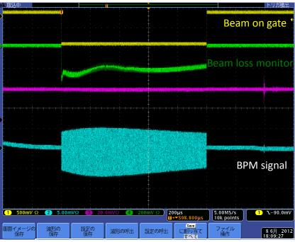
Beam acceleration with 1ms train (15pC/bunch) (Gun/SCRF RF feedback ON) 06.08.2012
