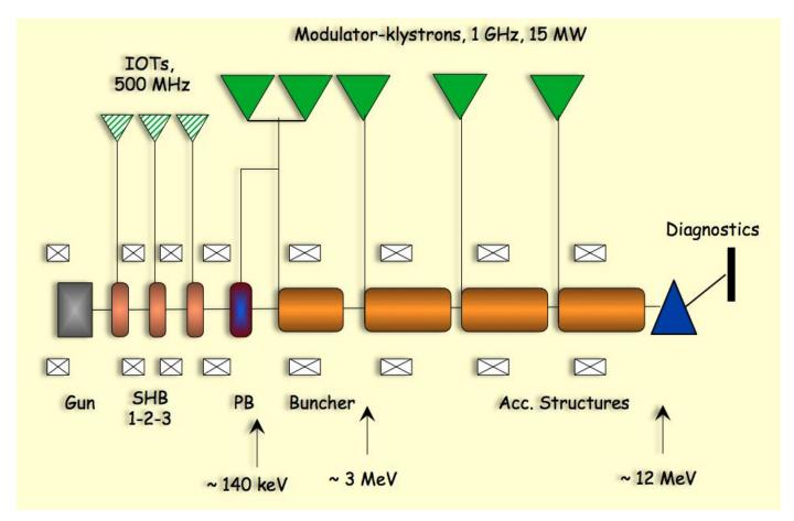
Gun, sub-harmonic bunching, bunching, three accelerating structures, 5 long pulse klystrons and modulators, diagnostics
