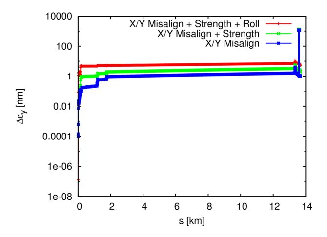
⇒ X/Y Offsets: Final average emittance growth is 1.06 nm (1.58 nm 90% c.l.) ⇒ Add Quad/Sbend Strength: Final average emittance growth is 2.01 nm (3.51 nm 90% c.l.) ⇒ Add Quad/Sbend Roll: Final average emittance growth is 5.36 nm (9.94 nm 90% c.l.)
