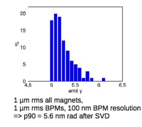
A trivial but important remark: Outgoing beam position jitter depends only on 27 our knowledge of BPM position and BPM resolution at the end of the loop!
