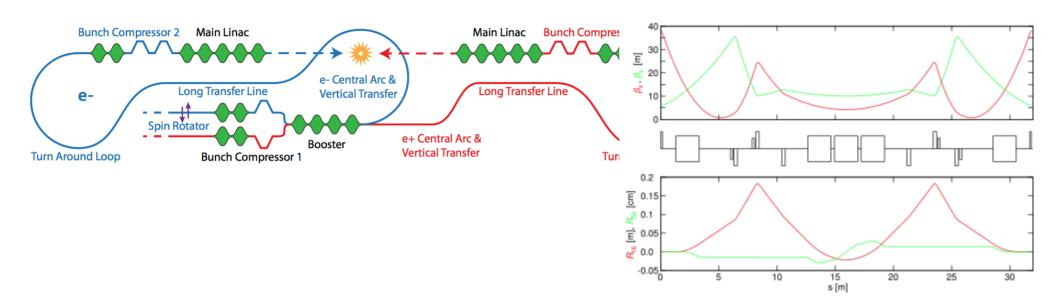
Each RTML consists of about 26.3 km of beamlines: 21km for each transfer lines; 2km for each turn around loop
