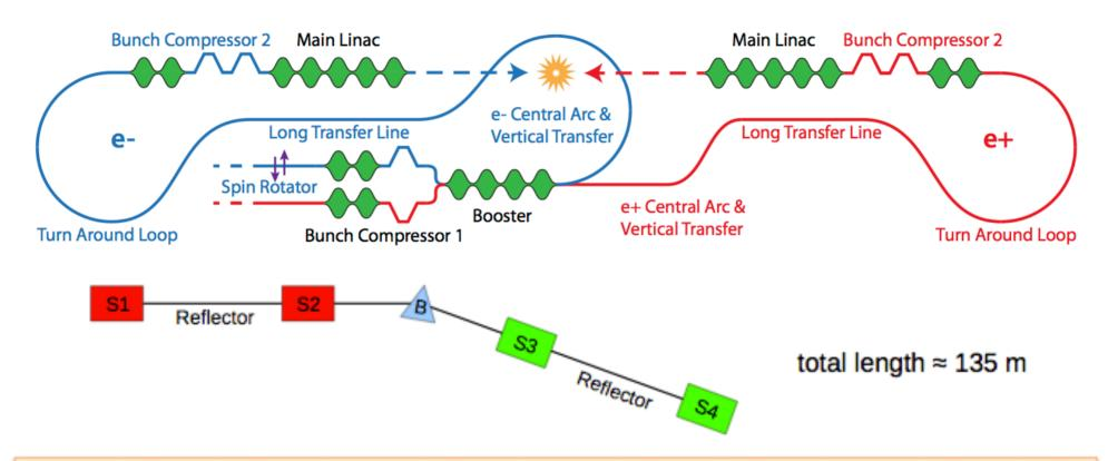
To avoid spin dilution the spin vector is oriented in vertical direction in the damping rings
