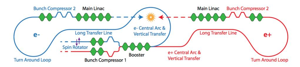
• Electrons and positrons share the same booster linac, from 2.86 to 9 GeV energy
