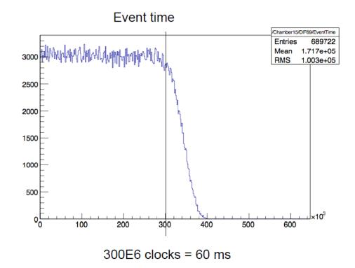
On 14/02 : memory depth = 60ms For this run : 7185 readouts in 3314 seconds ie 1 readout each 461ms And 4434 tracks found according to analysis configuration (5 pts per track)
