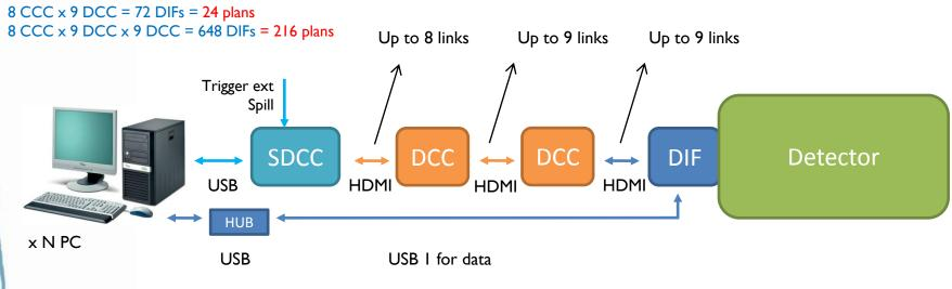
DCC : Data Concentrator Card SDCC : Synchronous DCC
