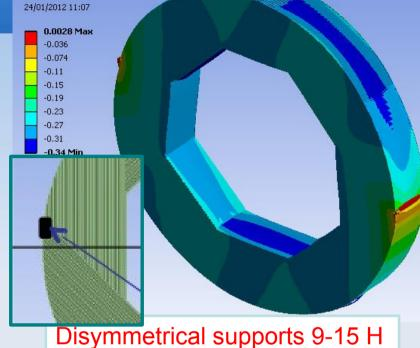
(Max deformation: 0.45 mm for position around 8-4h for support @ 4 & 8h)
