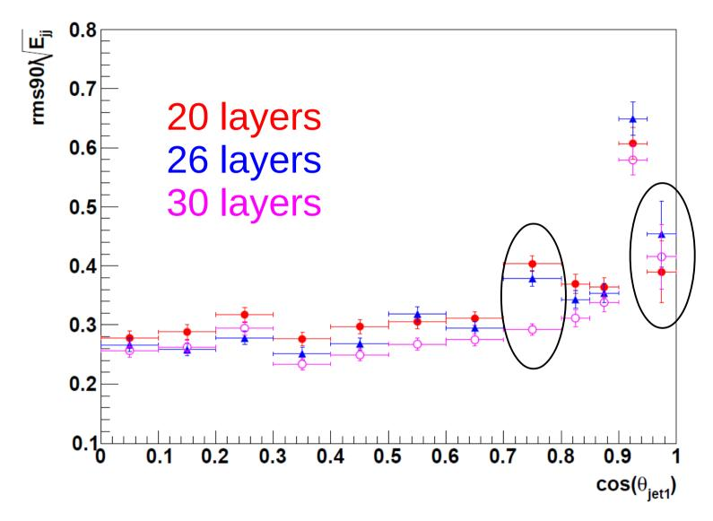
26 and 20 layer models have problems in barrel/endcap overlay, not seen for 30 layers Behaviour in forward looks a little strange...
