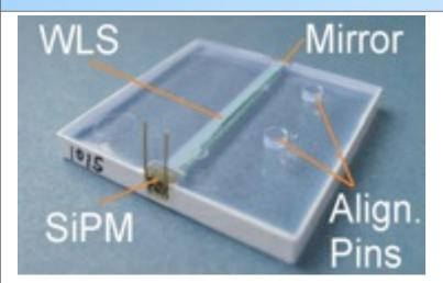
3 mm thick scintillator tiles integrated SiPMs "Lego" alignment Easy testing and characterization before installation
