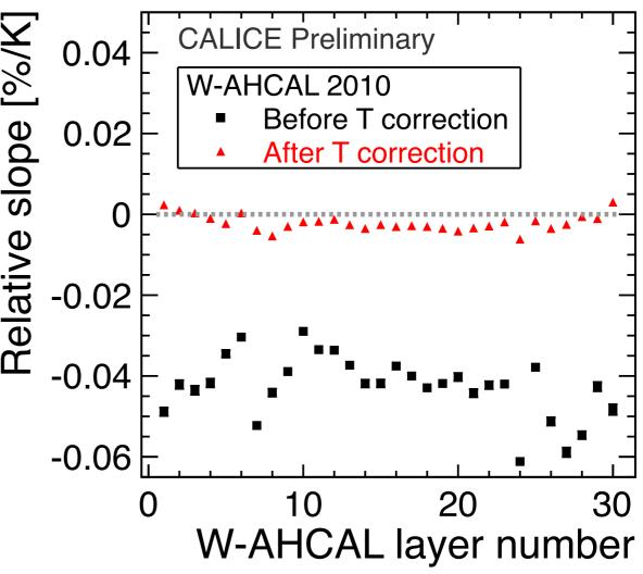
• With temperature monitoring (or using the intrinsic self-calibration of the SiPM, successfully demonstrated for T3B), this dependence can be corrected for to high accuracy over a temperature range far beyond what is expected in ILD
