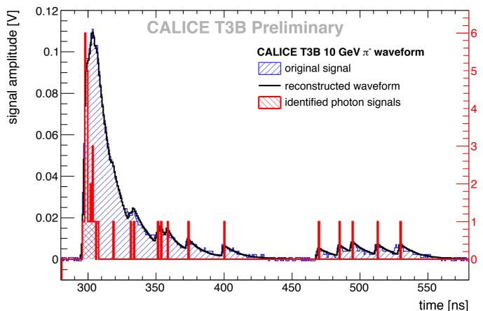
Signal on one tile, decomposed into individual single photon signals
