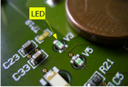
SMD LEDs embedded in PCB, one for each Tile: Easy, robust calibration
