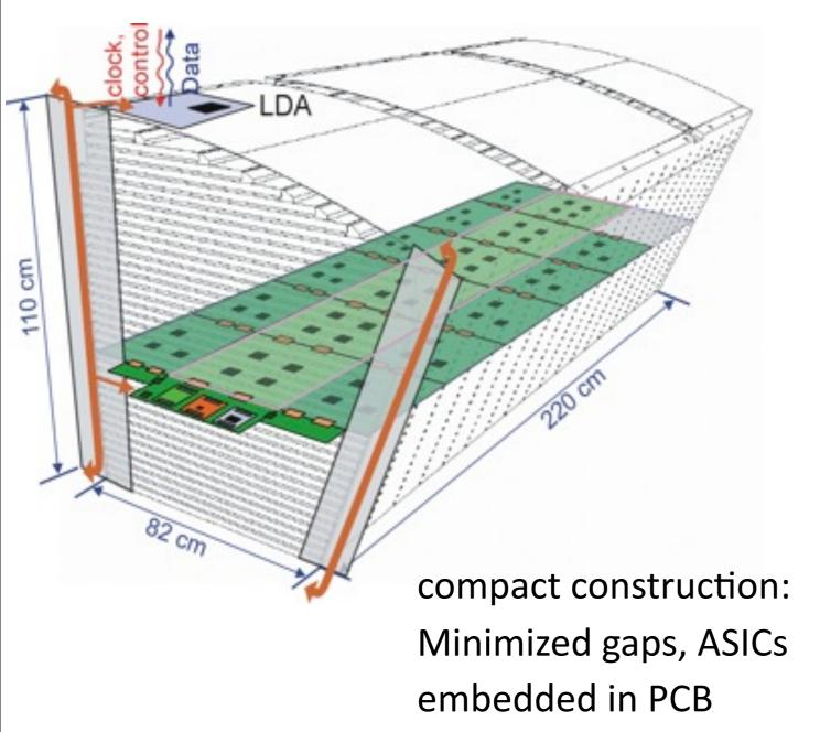
width of board and scintillator tiles can be adjusted in 1 cm steps to accommodate changing layer width
