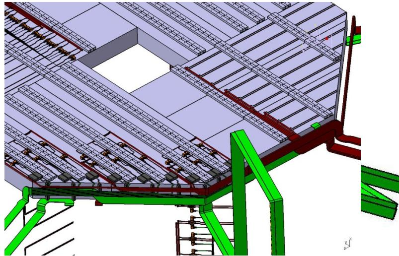
A solution with parallel or perpendicular rails / modules is better to allow free passage for cooling pipes & services
