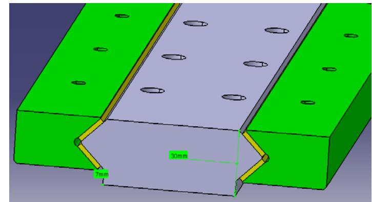
Finite element calculation to determine the stiffness of the rails : Wide / narrow
