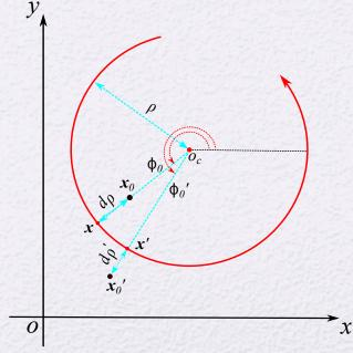
• The Kalman filter package, KalTest, is used for tracking. Helix parameterized in KalTest:
