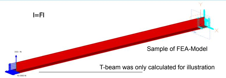
T-beam may have a buckling problem, the current model only provides basic properties. The next calculation will be done with an rectangluar or squared hole profile. Possible profiles will be selected with a max. deflection of f=10mm.
