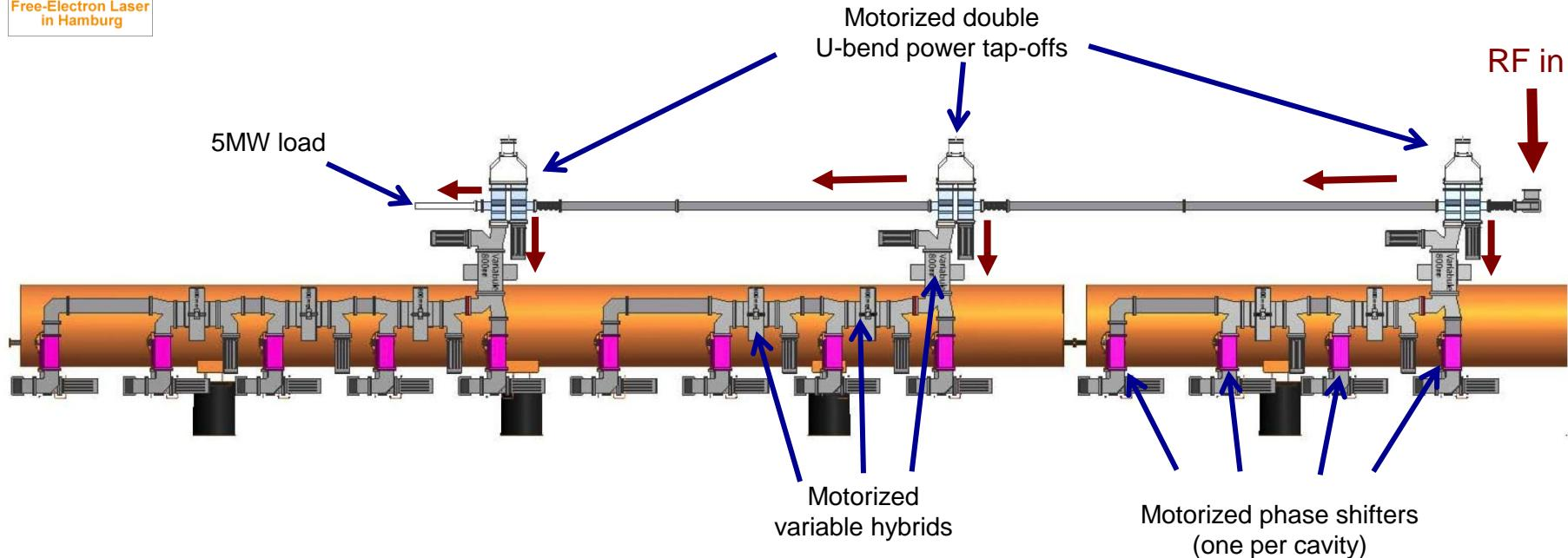
**KCS (RF source: one CTO per 3 cryomodules)**
