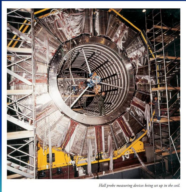
*Hall probe measuring devices being set up in the coil.*
