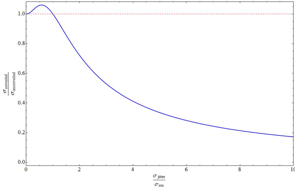
To achieve good jitter correction, the BPM resolution must be much smaller than the expected beam jitter.
