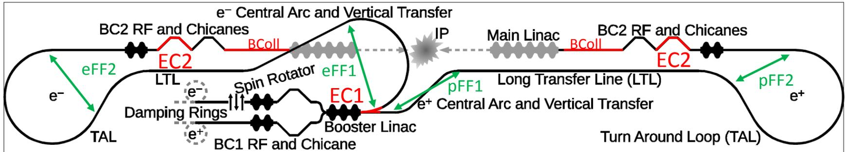
The  $e^+$  RTML has a chicane rather than a loop for the central arc; pFF1 will be different to the other FF systems.
