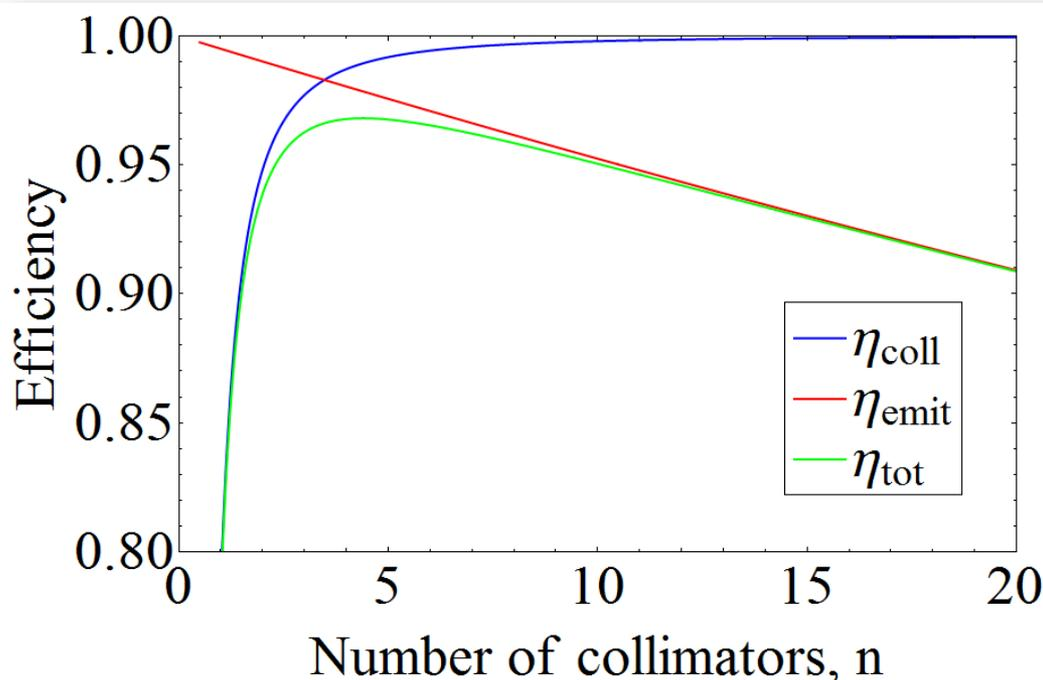
For the RTML betatron collimator parameters,  $\eta_{tot}$  is maximal when  $n = 4.4$
