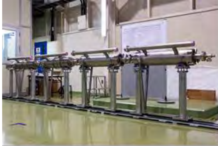
Figure 7-10: Completed S1-Global Module-C cavity string outside the clean room.
