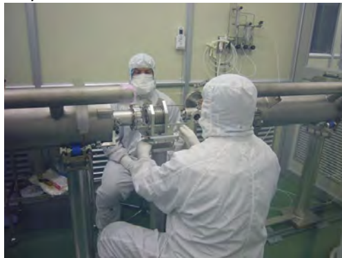
Figure 7-6d: DESY cavities aligned with the interconnecting bellows for string assembly.
