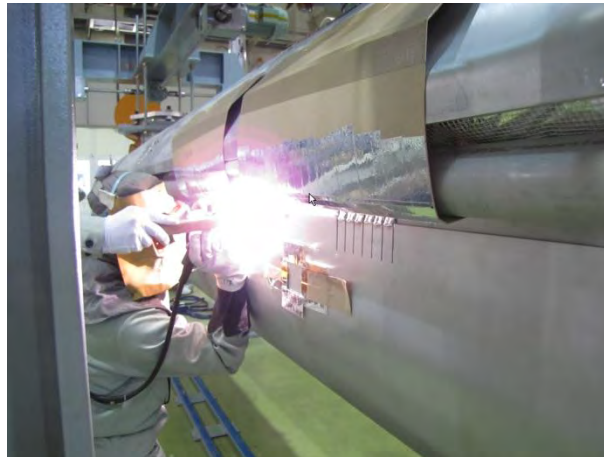
Figure 7-26: Staff member welding the lower 5 K shield to the upper shield.
