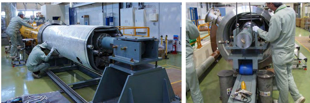
Figure 7-27: Staff member inserting the Module-C cold mass into the cryostat.
