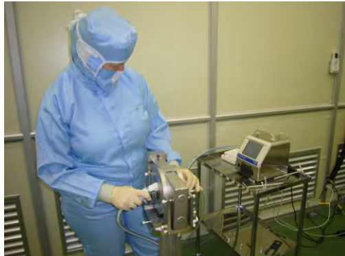
Figure 7-4b: DESY clean room technician cleaning the gate valve with ionized nitrogen.
