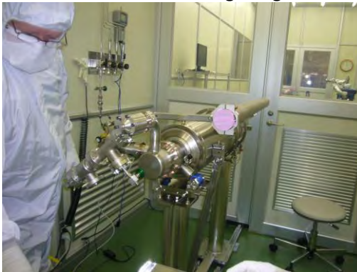
Figure 7-4c: FNAL clean room technician performing a pre-string assembly leak check on a cavity.
