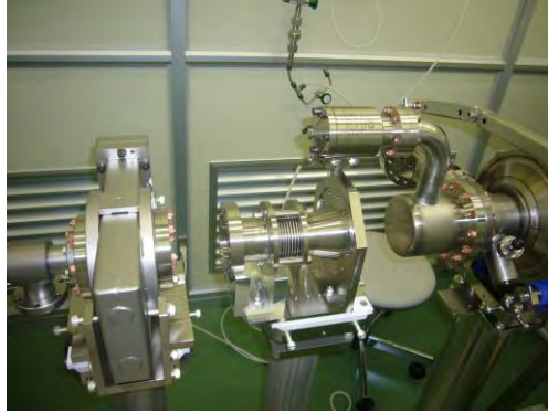
Figure 7-8a: Step-1 to Step-4 assembly with transition piece.
