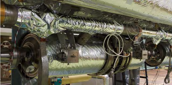
Figure 7-24: Attachment of the cavity-string to the GRP.
