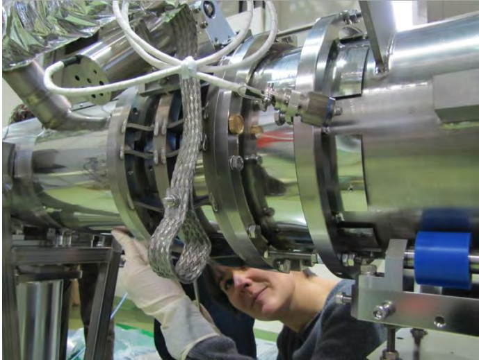
Figure7-23: Staff member assembling the magnetic shield on the FNAL cavity jacket.
