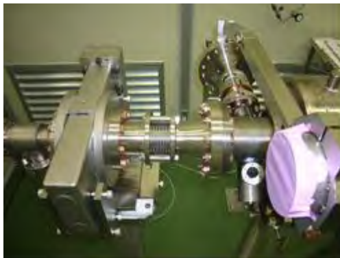
Figure 7-8b: Gate valve assembled with FNAL TB9AES-004 cavity via the transition piece.
