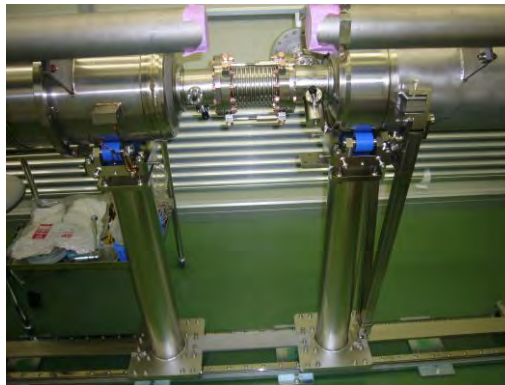
Figure 7-7: FNAL Cavity TB9ACC011 assembled with DESY cavity Z109 with long interconnecting bellows.
