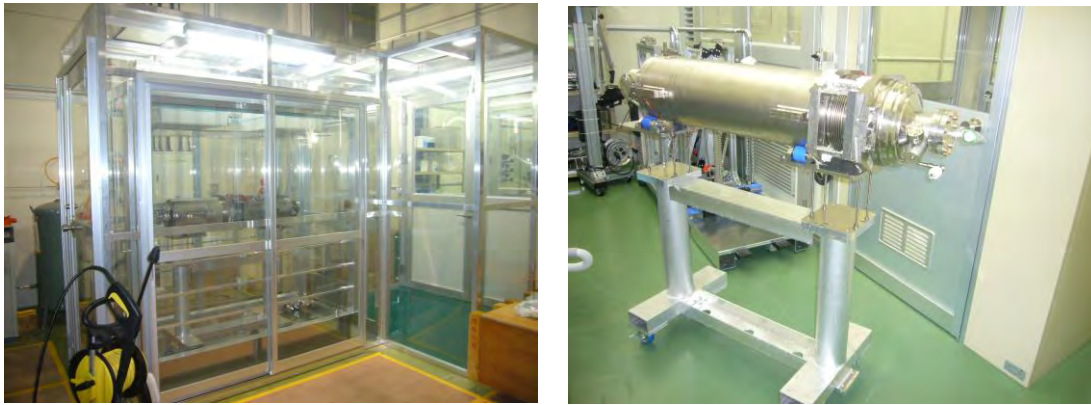
Figure 7-11: Cleaning booth at the entrance to the clean room (left) and cleaned cavity on a carrying cart inside the clean room (right).
