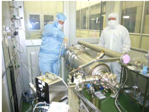
Figure 7-5c: Cavity moved into Class 10 area for string assembly.
