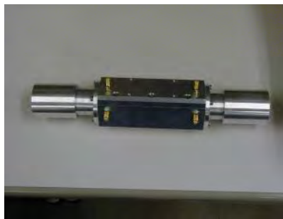
Figure 14-3: Drawings and photo of WPM pickup. Four strip-line electrodes with SMA connectors in both ends are installed in the aluminum body.
