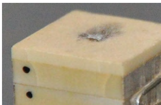
Figure 11.2.1-3: Fracture damage to the end plate of the piezo as a result of excessive shear forces.
