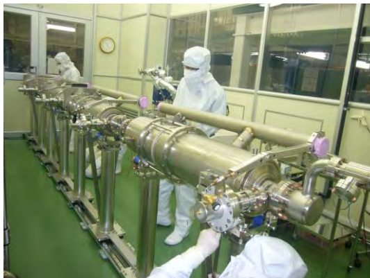
Figure 7-3 Preparation of cavities in Class 1000 clean room at KEK.
