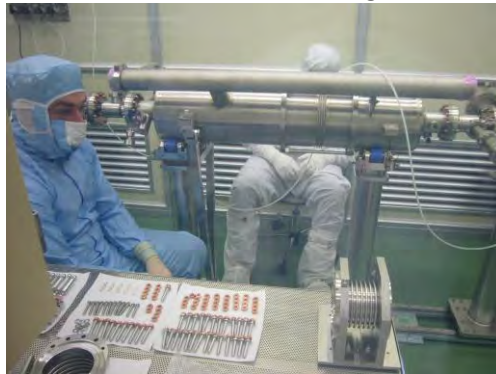
Figure 7-6c: Assembly hardware and bellows cleaned and ready for assembly.
