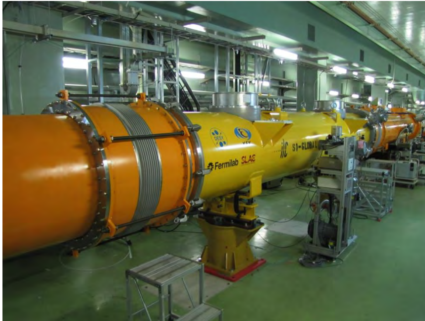
Figure 7-32: Connection of Module-C to Module-A.
