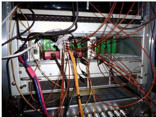
Figure 10-7: \mu TCA-based digital LLRF system during Stage 3.
