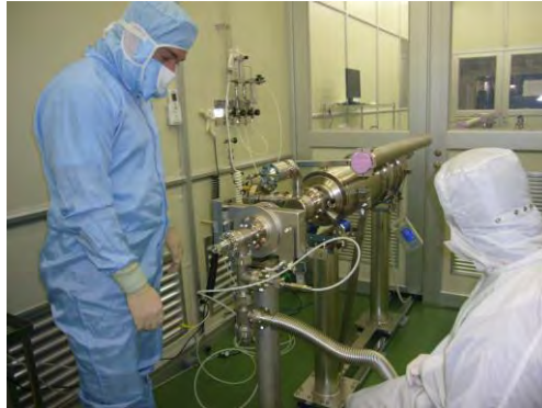
Figure 7-5a: Gate valve sub-assembly (step-1) leak check.
