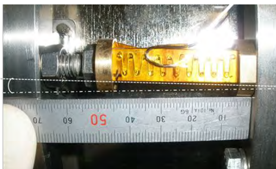
Figure 11.2.1-2: The brass end-caps holding the piezo-actuator. These were not well aligned with the result that shear forces were applied to the actuator stack.
