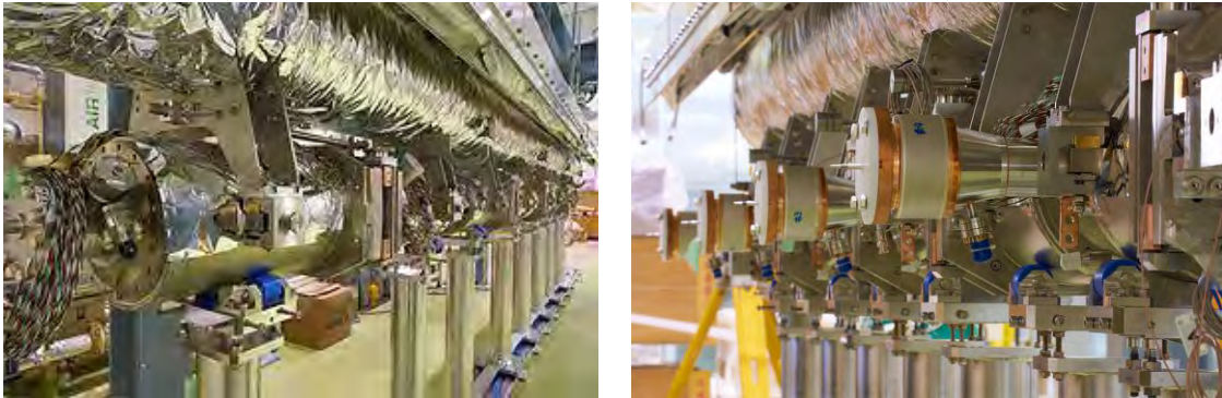
Figure 7-21: Attachment of movable supporting tubs for suspending the four cavities.
