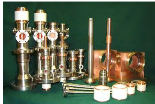
Figure 4-1: Schematic drawing of the TTF-III input coupler (left) and several components of the TTF-III input coupler (right).
