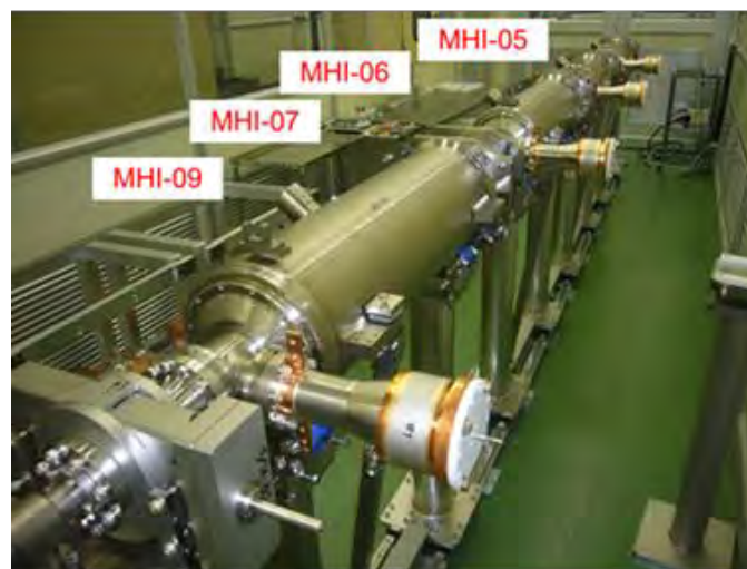
Figure 7-17: Completed string assembly of four KEK cavities in class-10 clean room.
