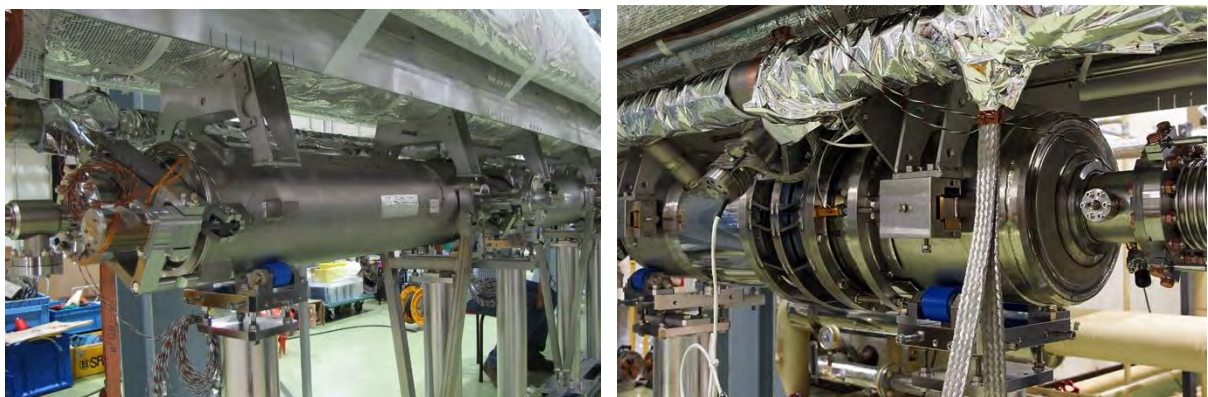
Figure 6-5: DESY (left) and FNAL (right) cavities assembled under the GRP.
