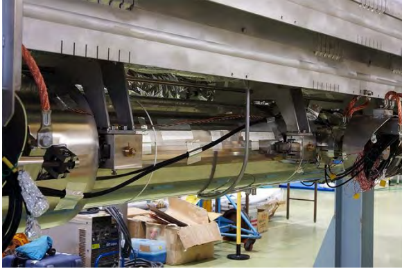
Figure 6-6: Magnetically shielded DESY (left) and FNAL (right) cavities.
