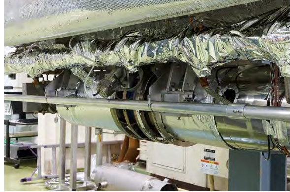
Figure 6-6: Magnetically shielded DESY (left) and FNAL (right) cavities.
