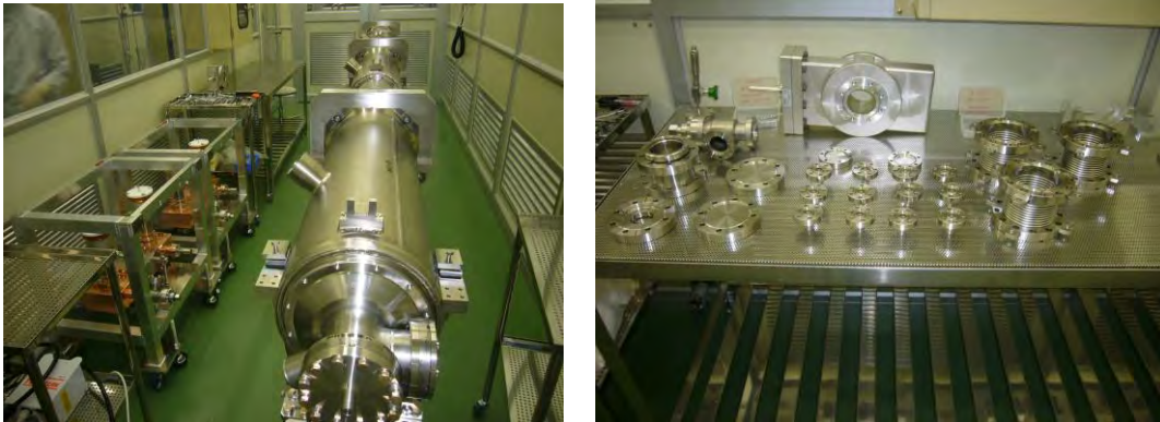
Figure 7-13: Preparation of cavity string assembly in class-10 clean room; four KEK cavities and four input couplers (left) and vacuum parts (right).
