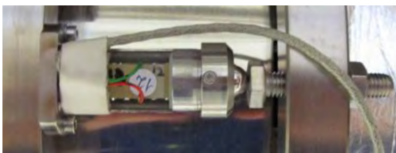
Figure 11.2.1-4: Fully encapsulated piezo-actuators installed on the FNAL CM2 cavities. Encapsulation prevents the transmission of shear forces to the piezo stack.
