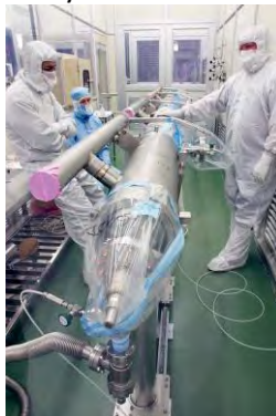
Figure 7-9: Fine leak checking of the assembled Module-C string.
