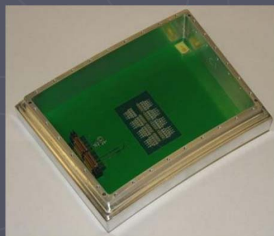
LP module with 8 Gridpix and a recorded event
