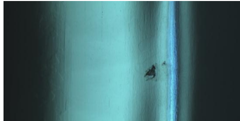
Cell 6 new defect 324 degrees
