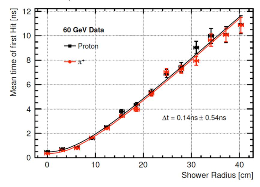
Compare protons and pions: No significant difference in timing profile seen
