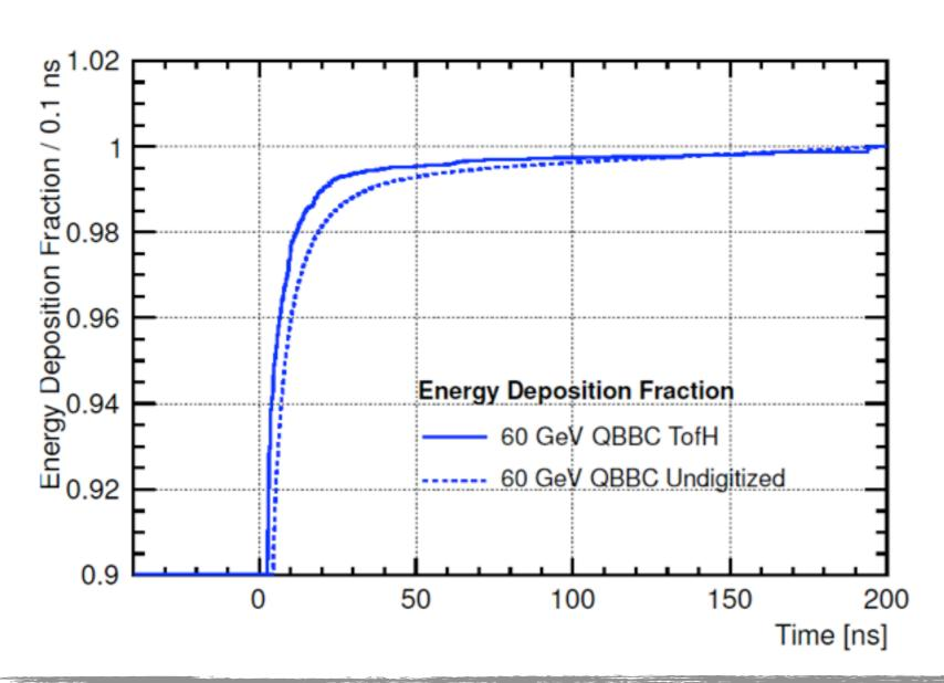
Time of first Hit T3B data is faster than the full calorimeter - but not dramatically
