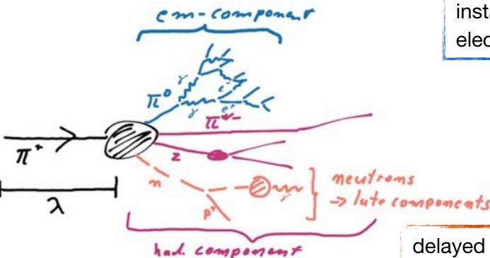
instantaneous, detected via energy loss of electrons and positrons in active medium
