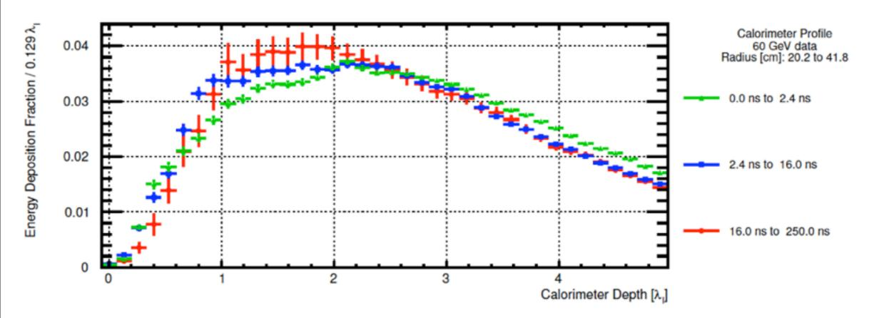
• The central part (dominated by EM - particles) drives the difference in shape - In the outer regions of the calorimeter the shower looks the same at all times...
